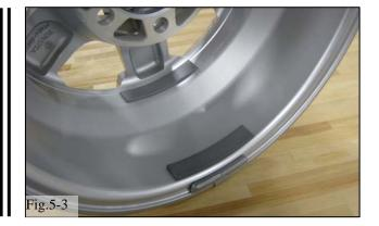
NOTE: Make sure that the tire bead and tool does not interfere with the main body of the sensor and the bead does not clamp the sensor.
