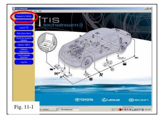
10. TPMS Transmitter ID Registration Perform ONLY when replacing sensors. Skip to step 12 if re-using same 20 degree Skip to sensors.
